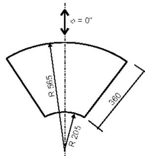
Figure 6 : Typical cross section of a damper
