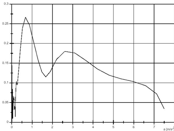
Figure 9 : typical curve representing the damper efficiency as a function of structure acceleration.
