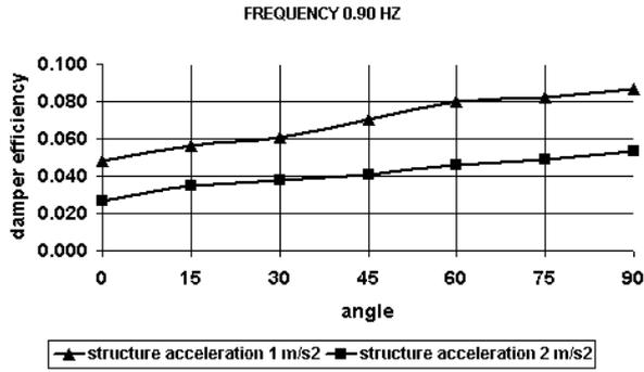
Figure 7 : damper efficiency versus angle of wave in the damper unit for an exciting frequency of 0.90 Hz at a different acceleration rate
