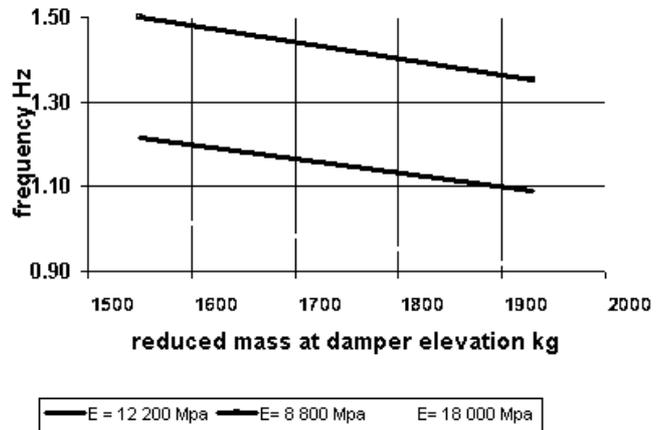
Figure 5: structure frequency versus reduced mass for different Young Modulus
