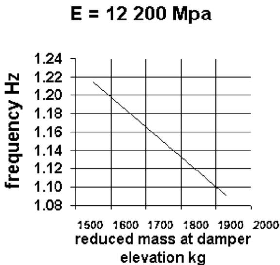
Figure 5:Structure frequency versus reduced mass
