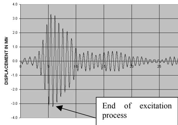
Figure 14: damping curve of the structure with a filled damper.
