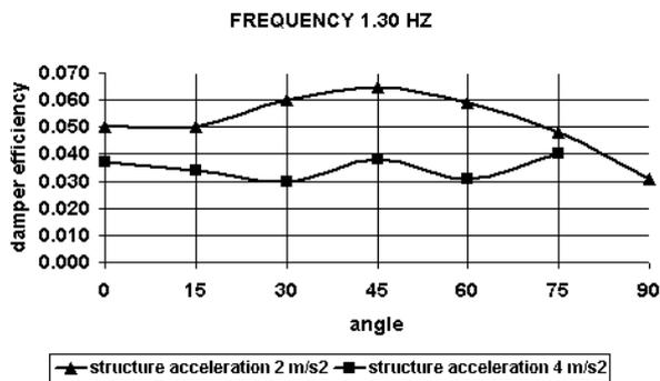
Figure 8 : damper efficiency versus angle of wave in the damper unit for an exciting frequency of 1.30 Hz at different acceleration rate
