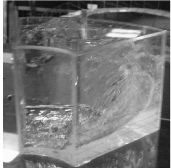
Figure 10: typical wave in a liquid damper
