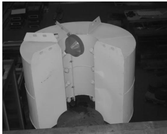
Figure 11: general view of the damper after manufacturing with nozzle for filling and internal space for ladder
